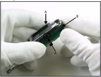
B. Carefully unattach the UI from the PWB.
