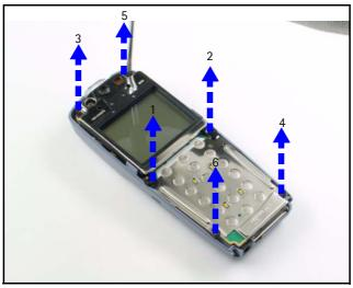
Note: During assembly, use the reverse order and use a torque driver with a torque of 25 Ncm.
